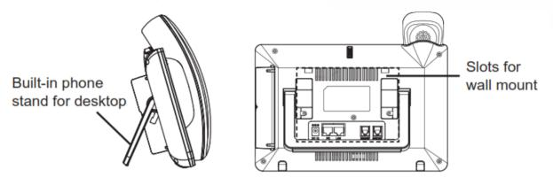
Figure 5: Built in Stand and Mounting Slots on GXV3370
