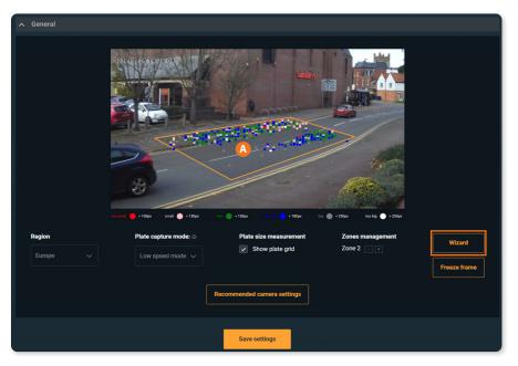
**Wizard** tool displays the statistic of the latest 1000 recognized plates sizes.
